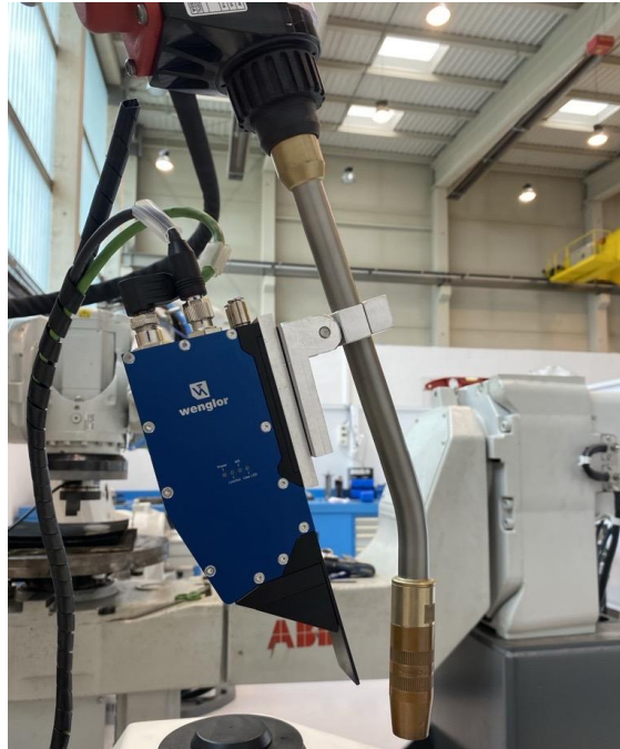
Figure 3. Wenglor profilometer integrated in the welding torch
