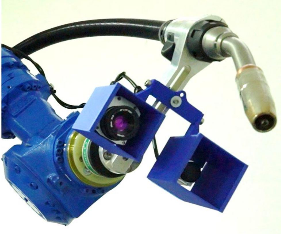
Figure 13: Initial sensor location - WAAM use case
